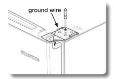
4. Remove the screw that holds the ground wire.
